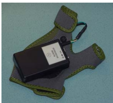
Figure 1: Data glove with battery and bluetooth transmitter box
