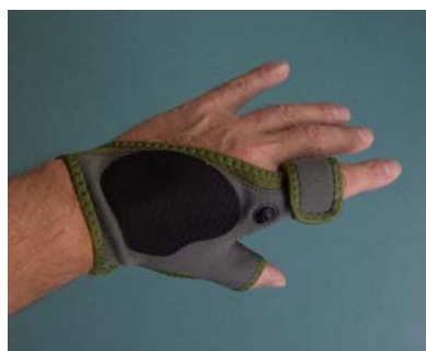
Figure 2: Data glove worn on the left hand without transmitter
